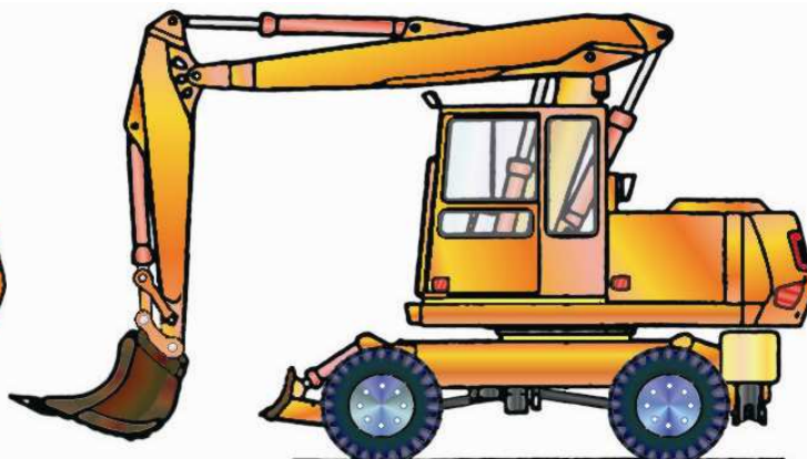
Fig. 2: Inverted position. Scoop hollow facing outwards
