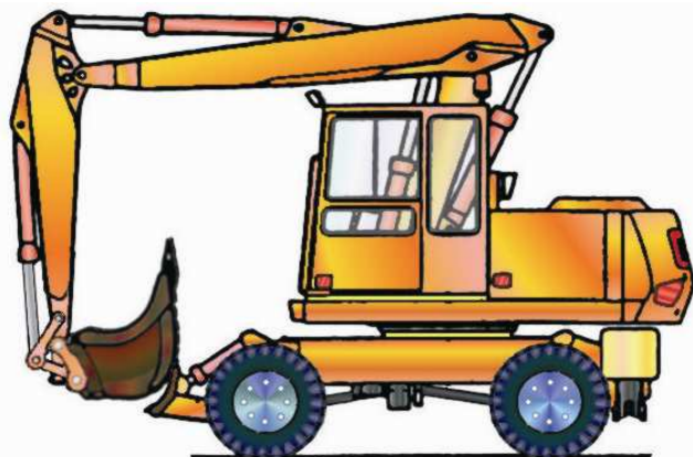
Fig. 1: Normal position. Scoop hollow towards operator's cabin
